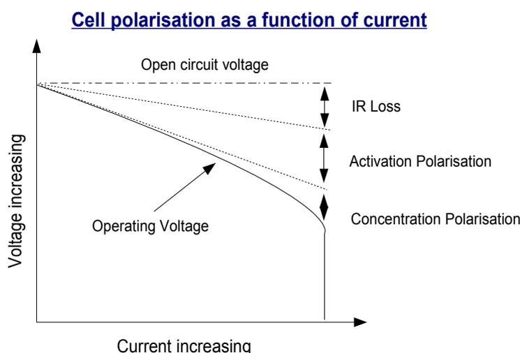
These polarisation effects cause losses at the electrodes which consume part of the energy and give it off as waste heat. Therefore not all of the theoretically available energy in the battery will be converted to useful energy.
