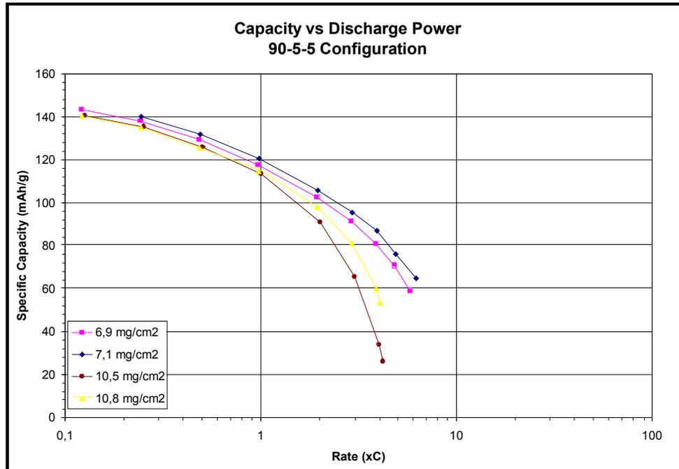
Therefore the generally quoted figures for the capacity of the LiFePO<sub>4</sub> material of 170 mAh/g are at low discharge rates of 0.1 C or less – this is a theoretical figure.
