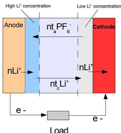
With the transport number for the Lithium cations  $t_c = 0.4$ ,  $n$  Lithium ions enter the anode compartment from the anode but only  $nt_c$  leave it and enter the cathode compartment, leaving a concentration build up of  $n(1 - t_c)$  or  $0.6n$  near the anode. Conversely,  $n$  Lithium ions leave the cathode compartment and are discharged as Lithium atoms in the cathode but only  $nt_c$  enter the cathode compartment, leading to a concentration deficit of  $n(1 - t_c)$  or  $0.6n$ .
