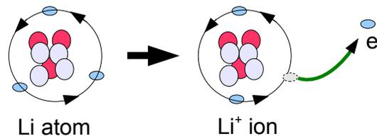
The Lithium ions then move through the electrolyte of the battery from the anode to the other electrode (the cathode) where they recombine with the electrons they originally lost which in the meantime have travelled through the outer circuit to drive the motor.
